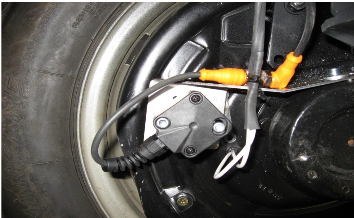
Mounting angle sensor on Dexter Torflex axle 12
