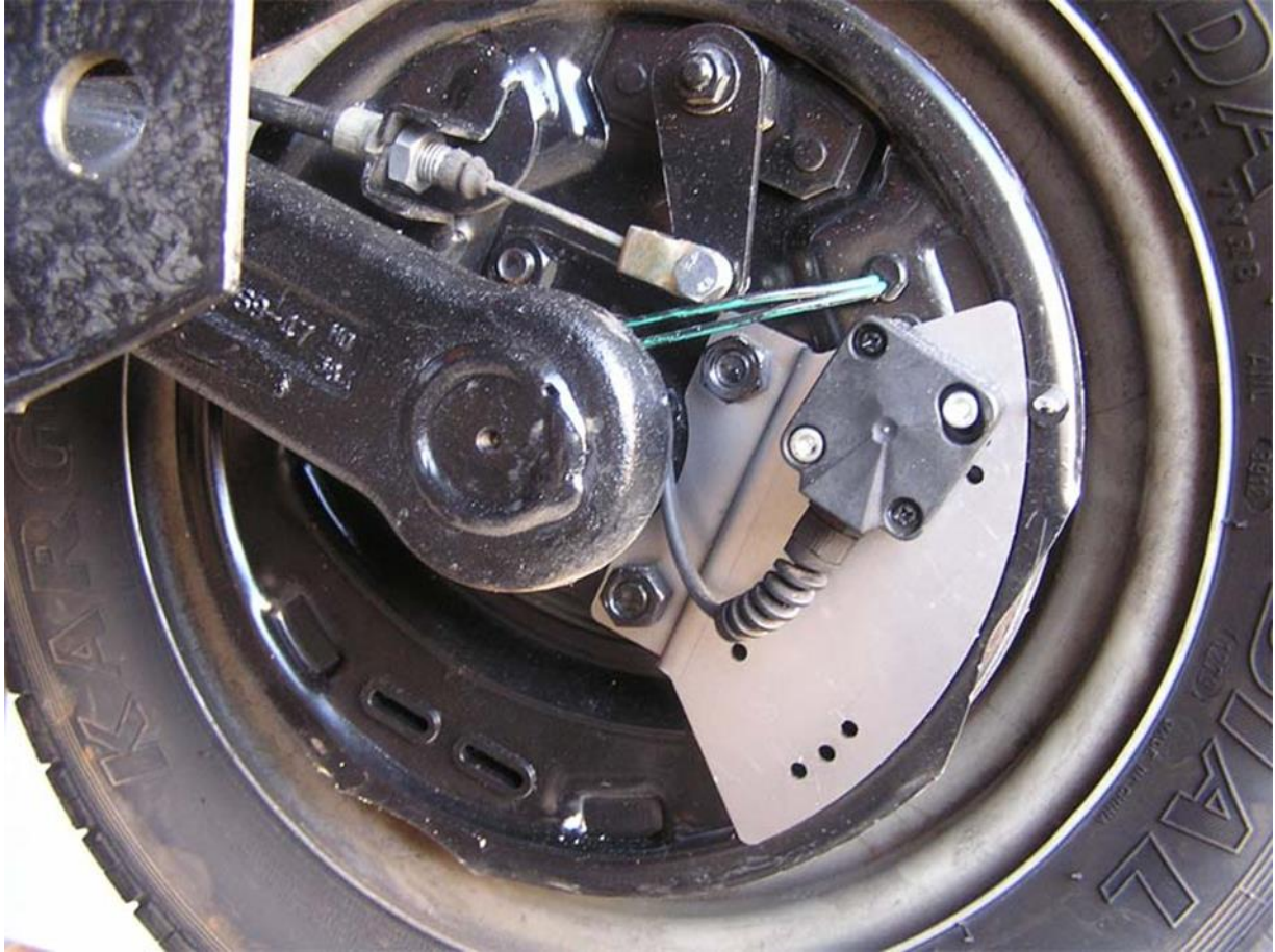
Mounting angle sensor on Dexter Torflex axle 10
